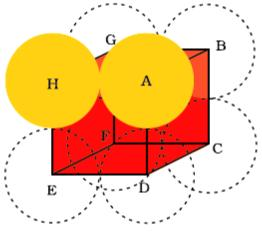
A simple cubic unit cell contains only one particle.
